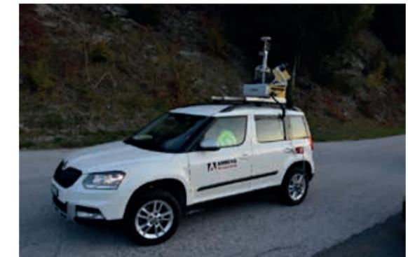
Abb. 3: Mobile Mapping System
